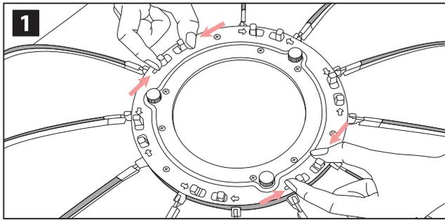
Close the Alpha Speedbox by simply releasing the rods from the speedring by squeezing on the 6 sets of tabs on the back of the speedring.
